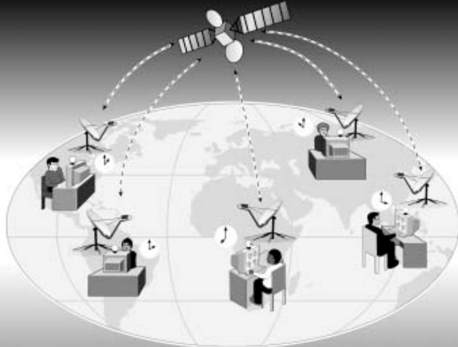
Two-way communication systems have more important uses. Here, antennas are able to both receive and transmit, providing two way services such as internet access, voice, data, or fax.
